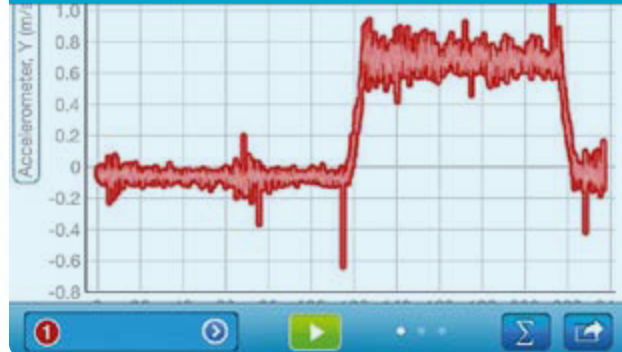
FIG.12 Acceleration vs. time in the y-direction without initialised offset
